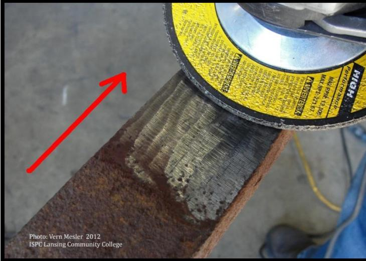
Select an area on the metal approximately 3” by 3”. Using a grinder with a 4” general purpose metal grinding wheel, grind in one direction. Do not grind in a back-and-forth or circular direction. Keep the grinder at 30 degrees.
