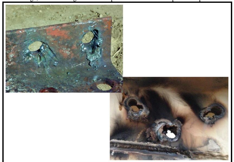
4) The operator continues cutting until most of the rivet is removed from the hole. At this stage, the remaining rivet can be punched out. This completes the process.
