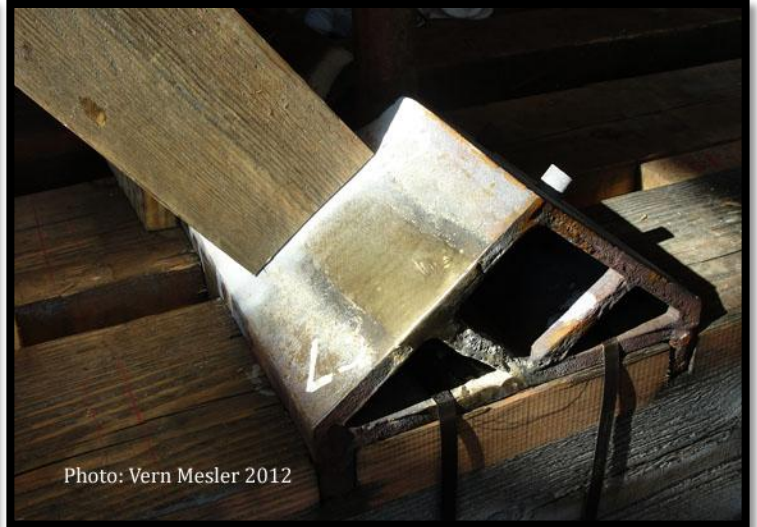
Lansing Community College braze welded repaired cast iron shoe
