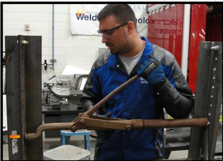
Mena uses the lever of the holder-on to apply pressure to hold the hot rivet in place. The process must be completed quickly so the rivet does not have time to cool.
