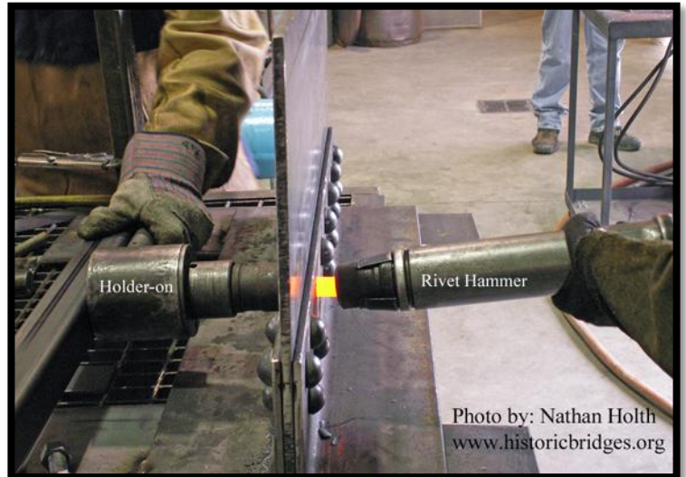
Commercially available pneumatic holder-on used with pneumatic rivet hammer in a demonstration at Lansing Community College, Lansing Michigan
