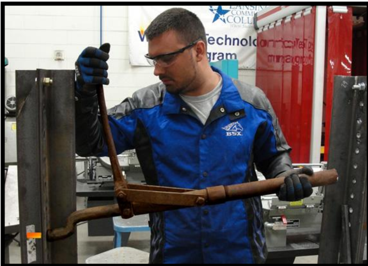
Craftsman-designed holder-on specialized for riveting at Fraser Shipyards, Inc. (Superior, Wisconsin) demonstrated by Adam Mena at Lansing Community College
