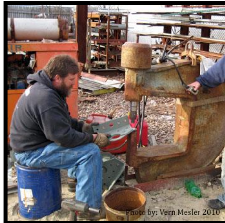
Tom Platt "Kooter" rivets section of a bearing end pad with Nels' 100-ton C-frame hydraulic press
