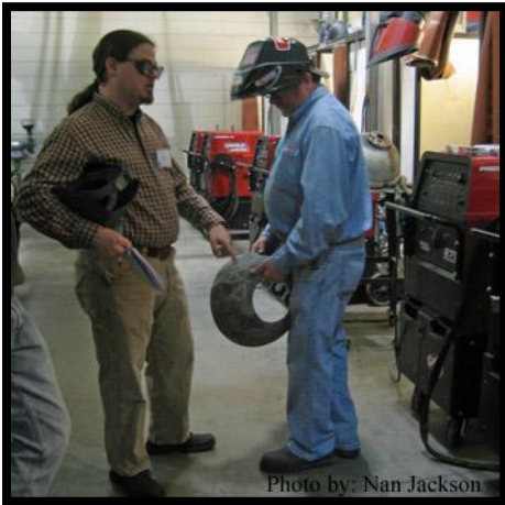
Photo by: Nan Jackson Roy Bailiff reviews the repairs made on an 1895 cast iron flange repaired with the SMAW process
