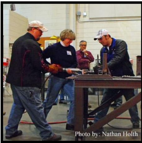
Roger Morrison and Adam Mena assist a workshop attendee in driving a rivet.
