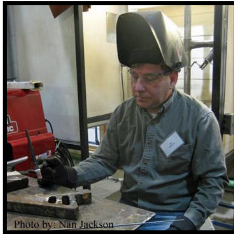
Photo by: Nan Jackson Bill Eggleston demonstrates welding cast iron with the GTAW process
