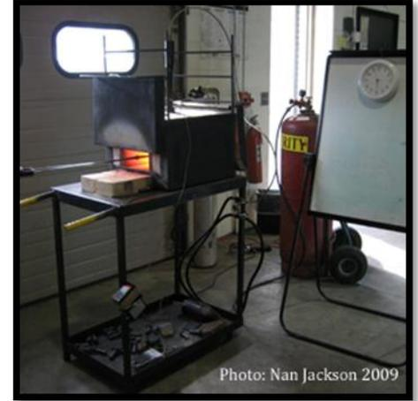
Temperature gauge is attached to the forge and a clock is handy for recording temperatures at one-minute intervals after the rivets are placed inside.
