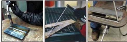
Flux Cored Arc Welding (FCAW)    Shielded Metal Arc Welding (SMAW)    Padding Section Loss with SMAW
