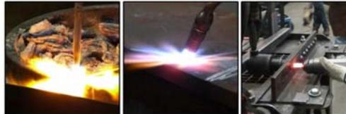
Braze Welding    Flame Straightening    Field Riveting
