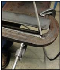
Shielded Metal Arc Welding
